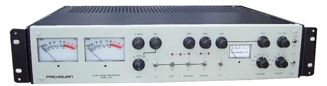
A single-ended noise suppressor designed to eliminate or reduce noises due to imperfections in and damage to sound recordings in all analog audio media and their digital reproduction, including cylinder, disk, film wire and tape recordings, both monophonic and stereophonic
